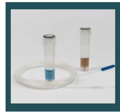
The ParaScope Protein Test Kit has been designed to allow the quick and reliable detection of residual proteins left behind inside endoscope channels. The long swabs provided are simply pushed down the length of the channel, removed and then swirled for 10 seconds in the liquid, to provide a clear and almost instantaneous result.
